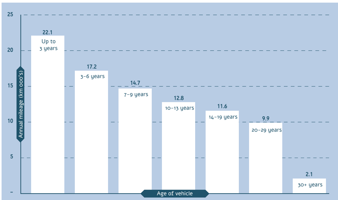
Figure 11: Annual vehicle mileage in thousands of kilometers as a function of vehicle age (2016 data)
